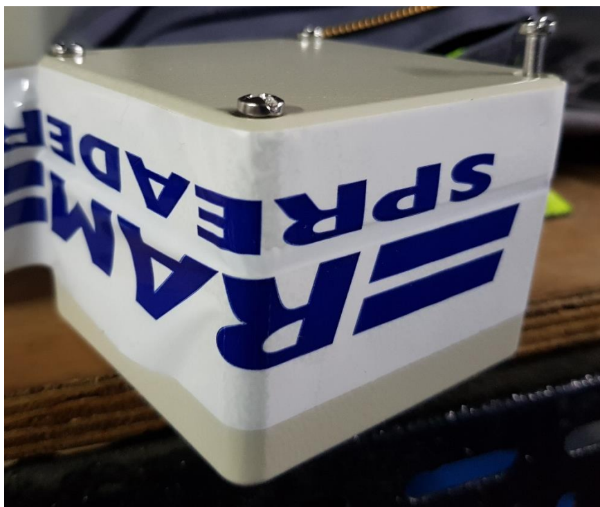
Figure 6 Brittle plastic tape sealing upper and lower part of electronic box.
