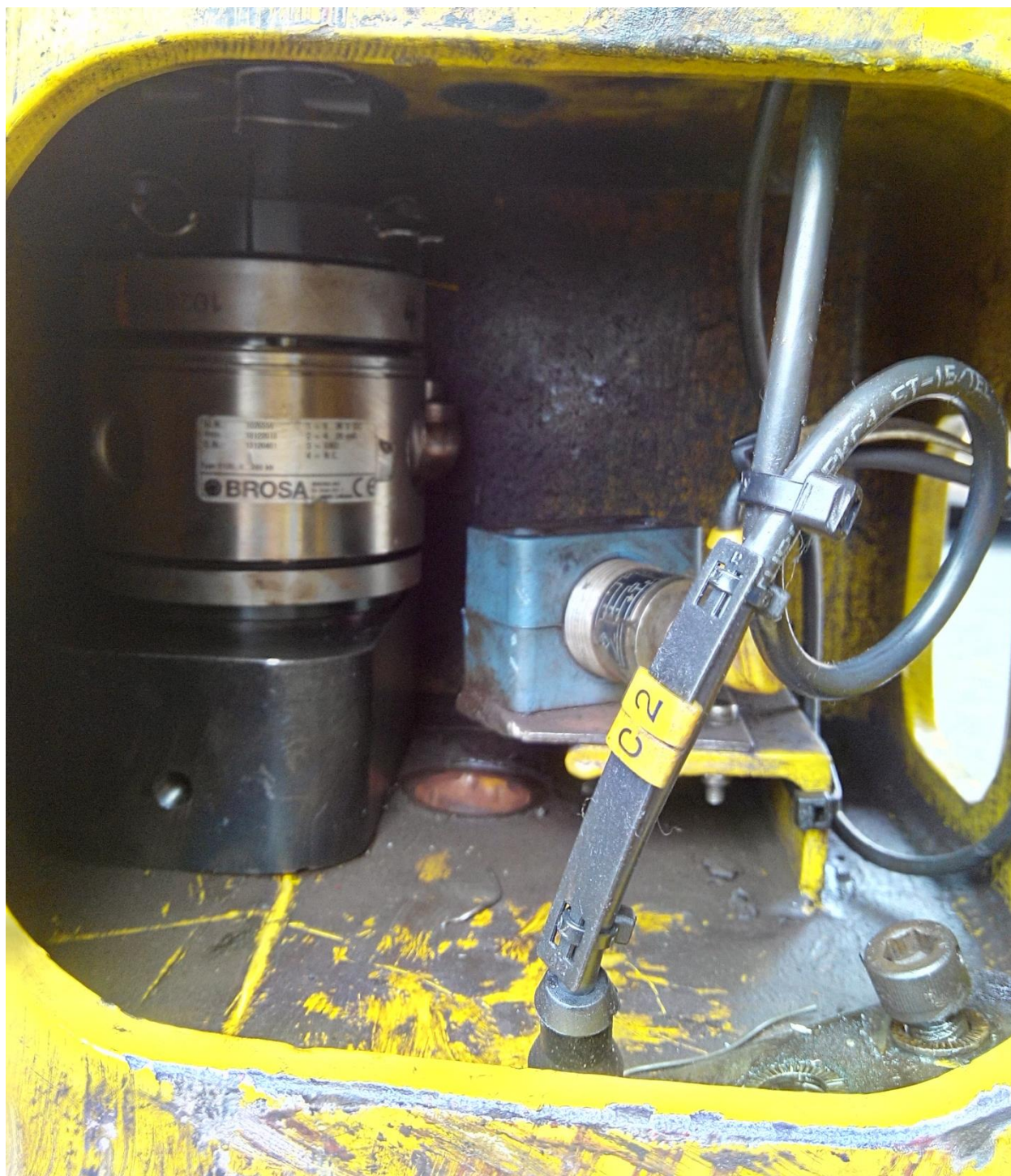
Figure 5 Load cell mounted inside spreader
