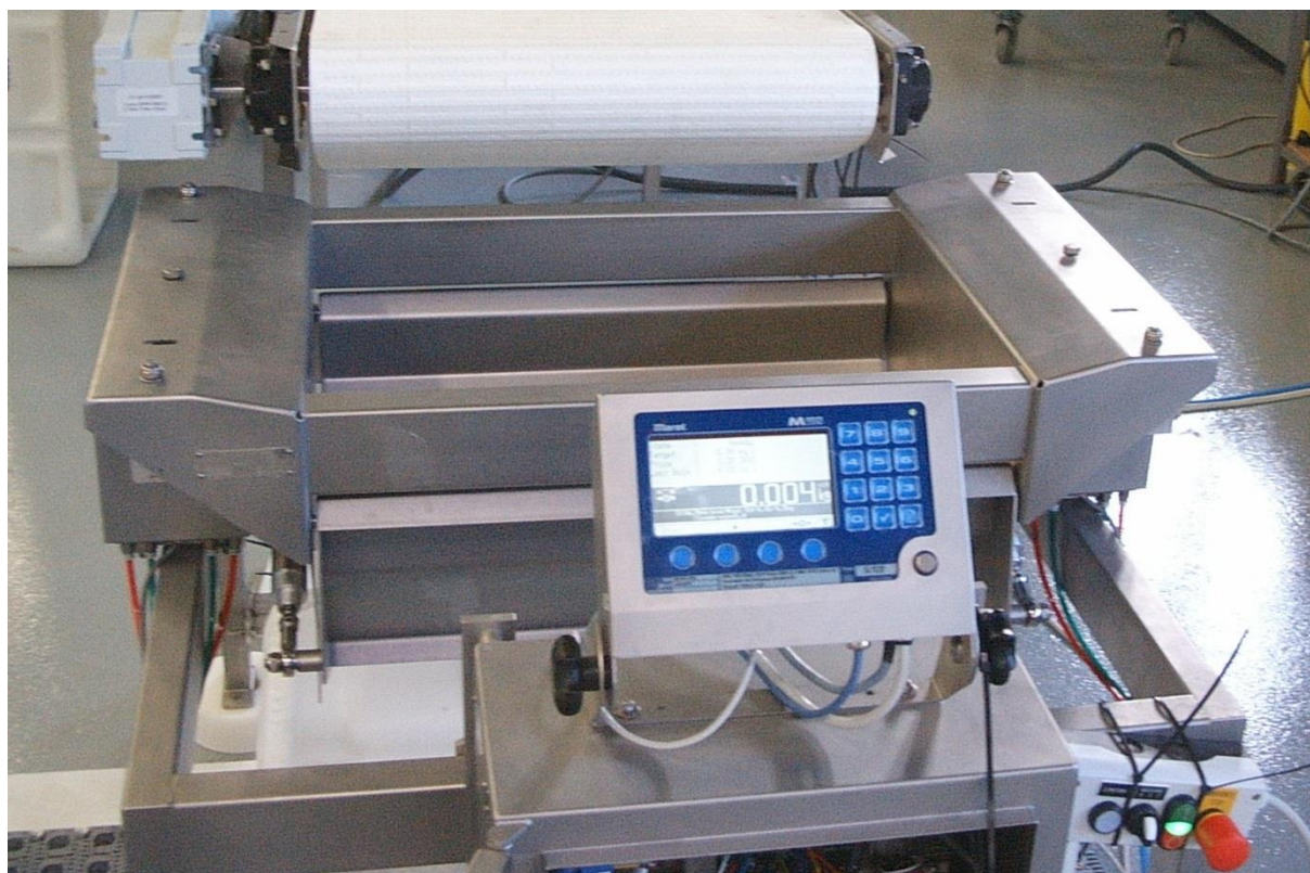
Figure 3 M2200-P02-HOP-xxxxx with 60 kg hopper load receptor.
