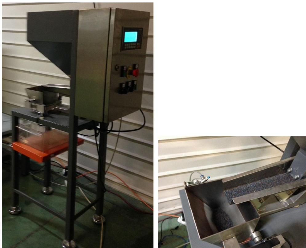
Figure 3 Example of a BX30 Total discontinuous totalizing automatic weighing instrument.
