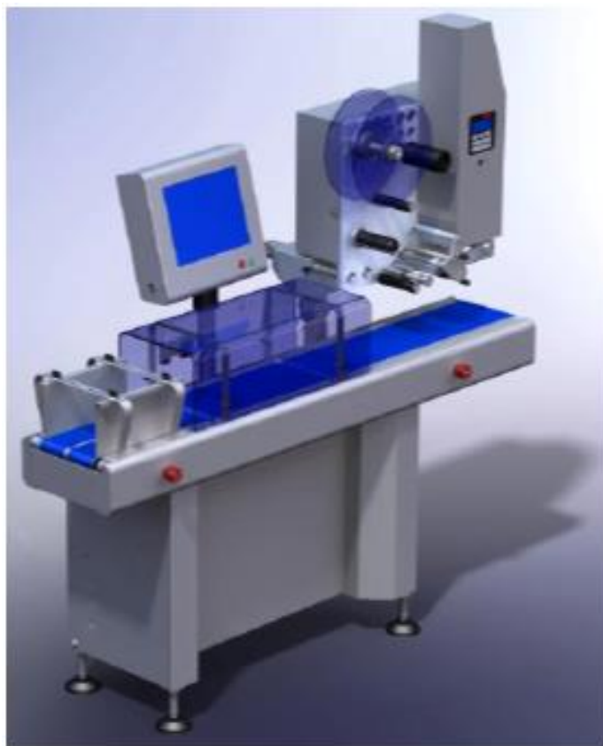
Figure 1 9000 series weighing instrument with top labeller
