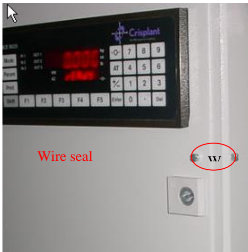
Figure 8 Sealing of Display Unit
