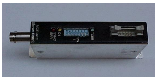
Figure 4 Digital Load Cell Module Type: MCE9610 or MCE2010
