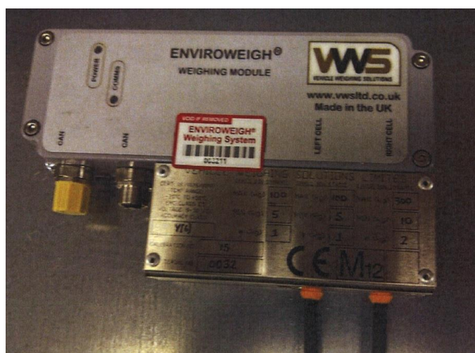
Figure 8 Labelled weigh control enclosure
