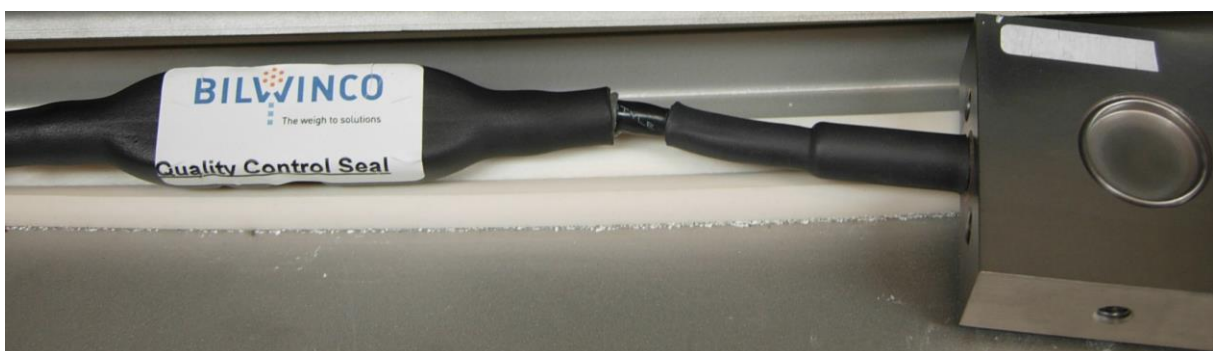
Figure 5. Sealing of load cell cable connector
