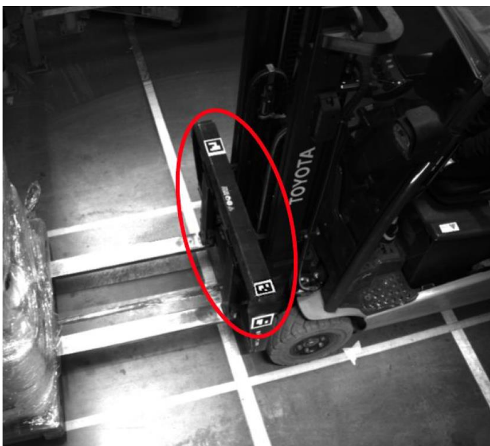
Figure 6 Example of ArUco marker placement on forklift.
