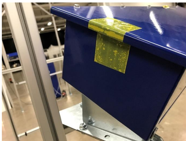
Figure 8 Sealing of stereo camera.
