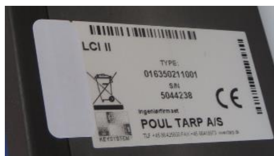
Fig. 2c , Indicator sealing example
