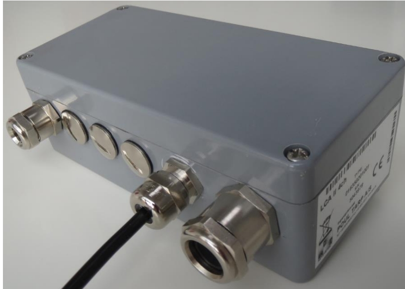
Fig. 1a, Load Cell Amplifier enclosure
