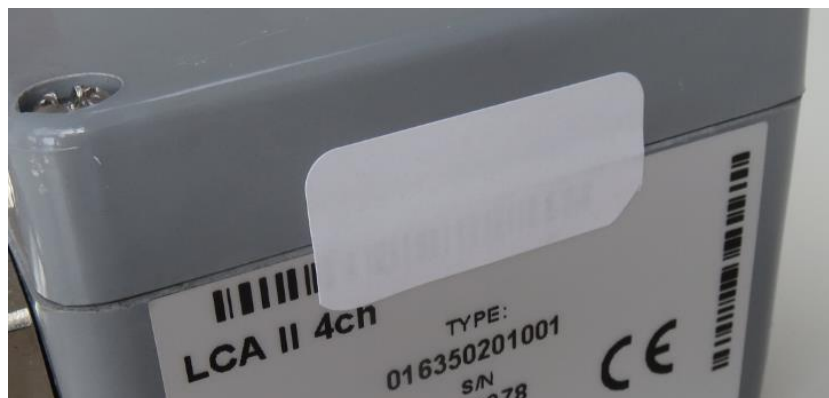
Fig. 1c, Load Cell Amplifier sealing example
