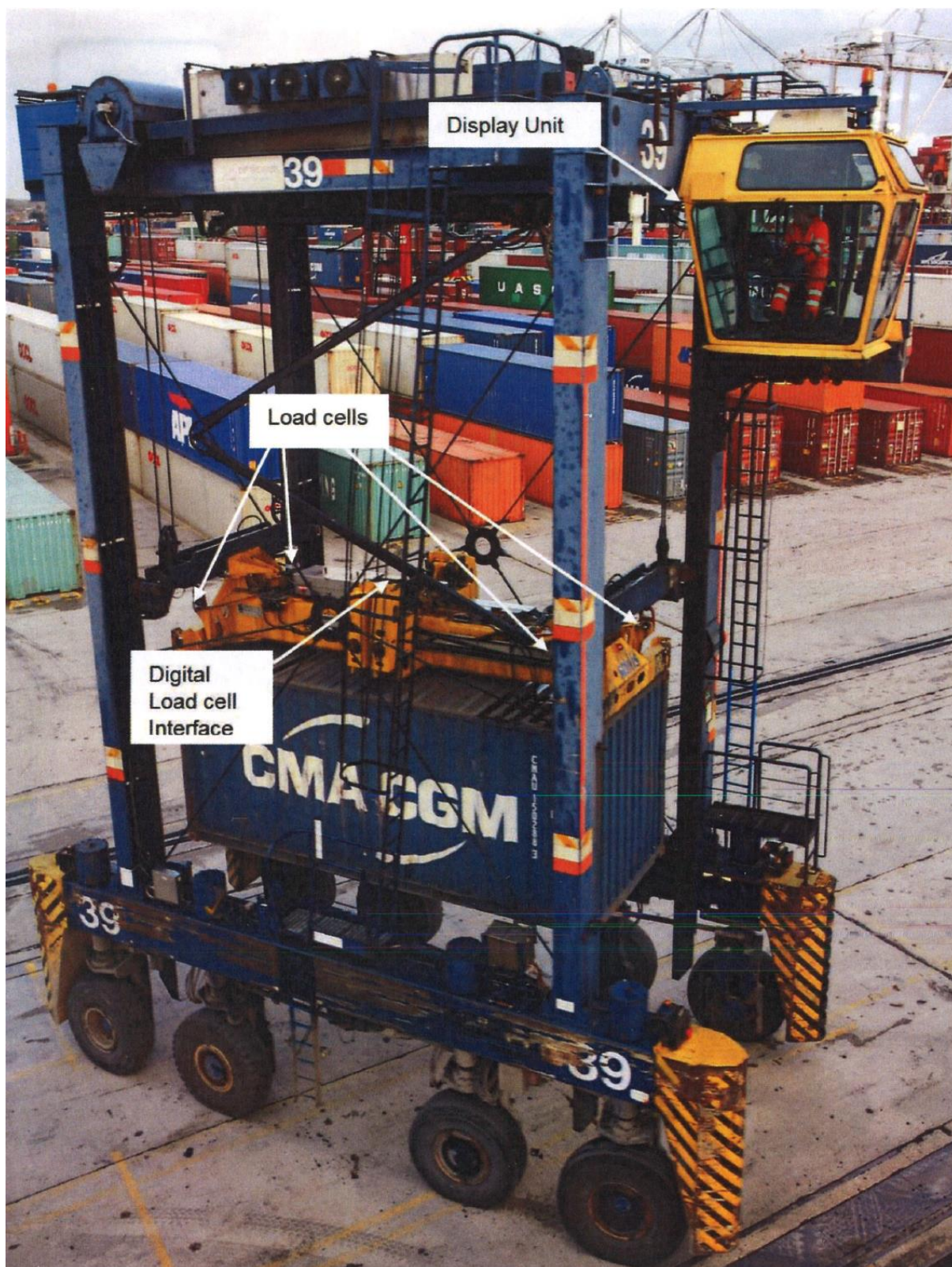
Figure 3 Typical spreader configuration
