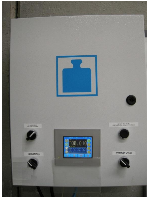
Figure 1: Control rack with operator's panel on front and weighing transducer and PLC inside
