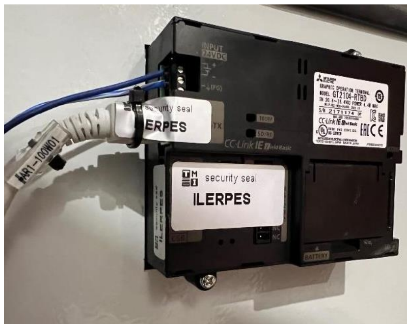
Figure 11: Sealing of GT2104-RTBD and its interfaces
