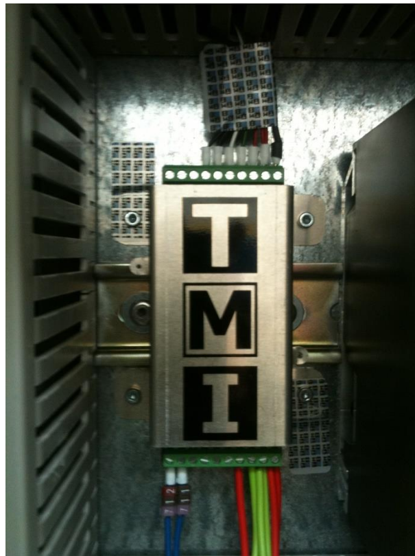
Figure 6. Sealing of LDU 78.1 weighing transducer, against removal and its load cell cable,
