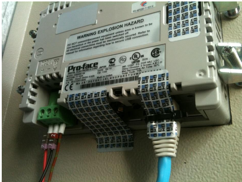
Figure 10: Sealing of AGP3200 / GP4201-T and its interfaces
