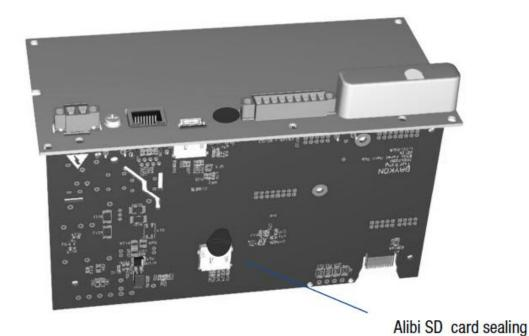
Figure 2 Sealing of FT-113 Fill indicator with brittle sticker.
