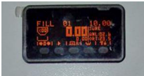
Figure 1. ECI weighing controller for automatic gravimetric filling instrument.
