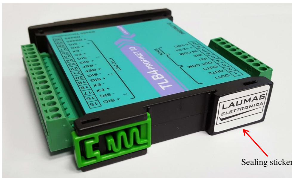
Figure 14 Sealing of TLB4 indicator.
