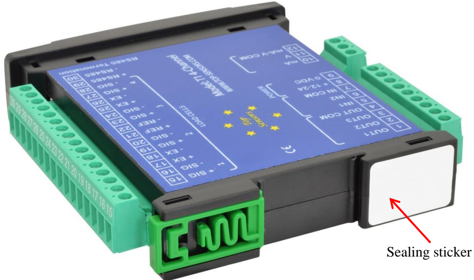
Figure 14 Sealing of Top-Sensors T1-4 indicator.
