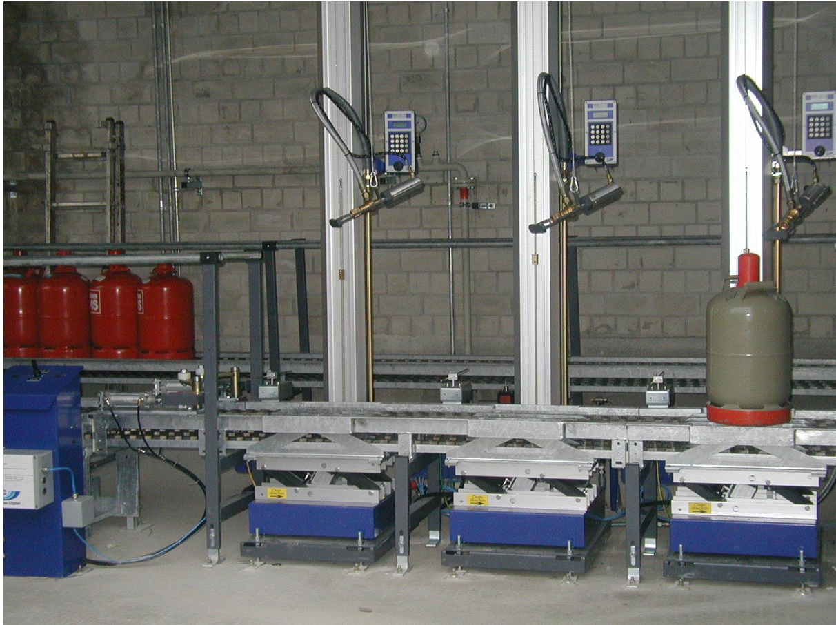
Figure 4 Inline ECS60 Filling Machine with check weighing.
