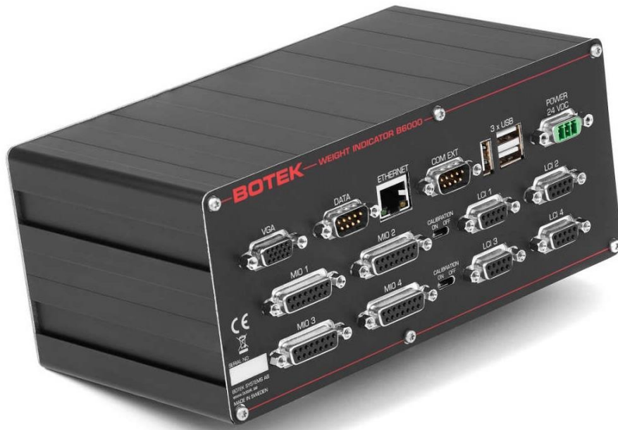
Figure 5 B6000 rear panel – with 4 scale channels
