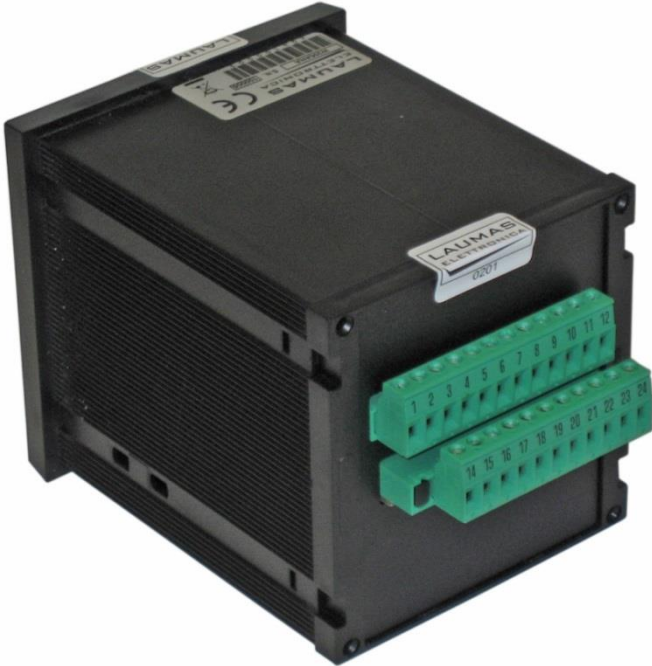
Figure 2 Sealing of W200 enclosure.
