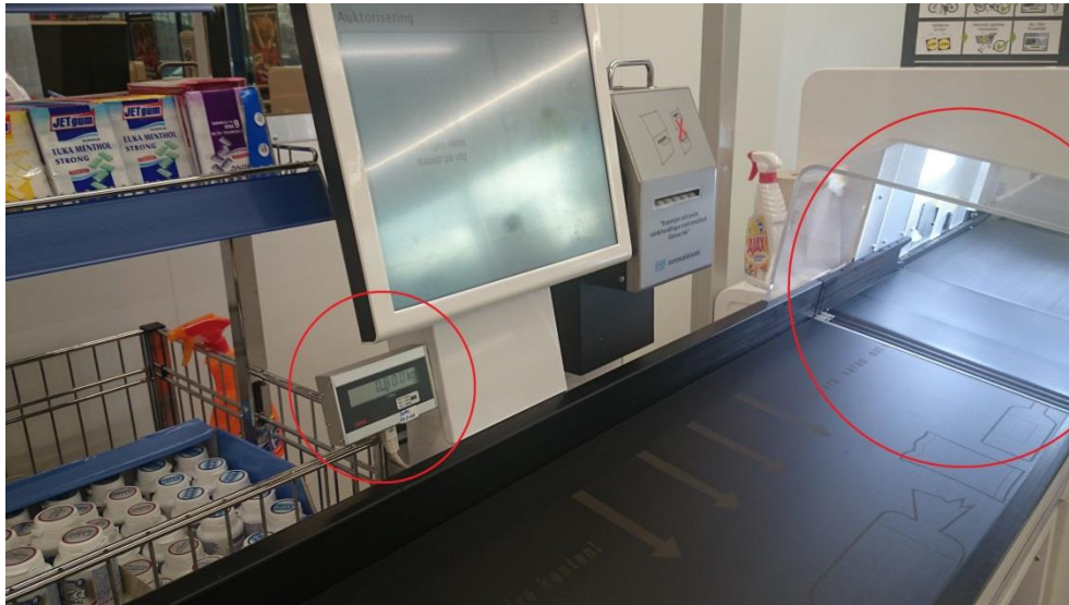
Figure 1 Example of the static weighing automatic checkweigher built into a self-service cash register line.
