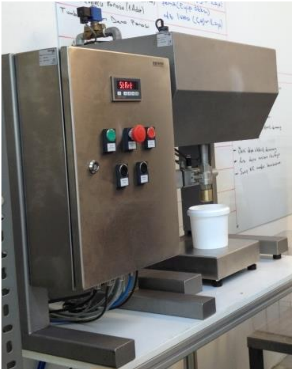
Figure 4 FT-10 Fill AGFI with platform load receptor for mode net filling
