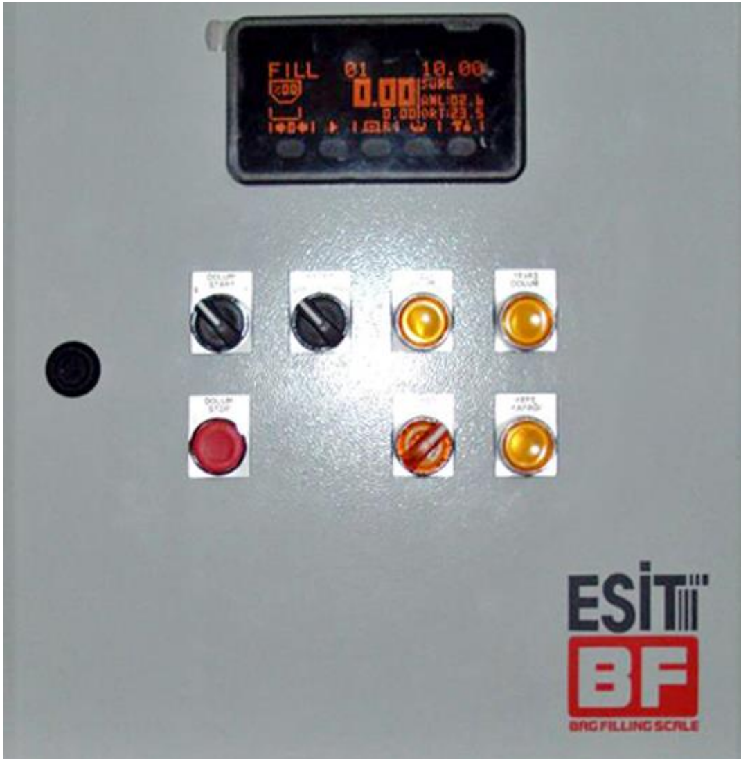
Figure 1. Control box for ECI automatic gravimetric filling instrument model BF with panel mounted ECI weighing controller.
