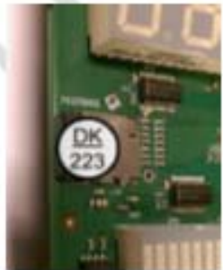
Figure 2 Sealing of the \mu SD-card for Alibi memory data.
