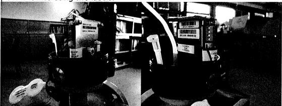
Furthermore the JTAG connector is sealed with an additional label:
