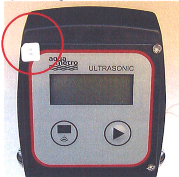
a) Sealing of electronics
