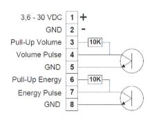
When Pulse Interface type 66-99-143 is connected to power supply or battery, the unit is placed on the meter, and the meter is in test mode, the following pulses are transmitted:
