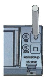
In order to access test mode the "TEST" seal (S) on the back of the meter must be carefully broken with a screwdriver and the contact points behind the seal short-circuited with a short-circuit pen or a screwdriver.
