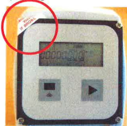
a) Sealing of electronics
