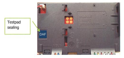
Close the Calculator securing that no wires are jammed by enclosure parts and rubber sealing.
